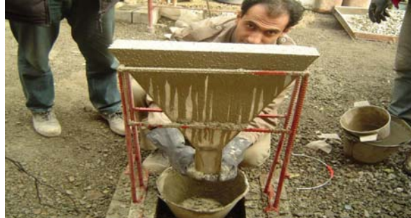
Figure 2. V-Funnel tests apparatus
