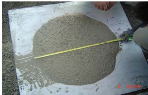
Figure 3. T-50 tests apparatus
