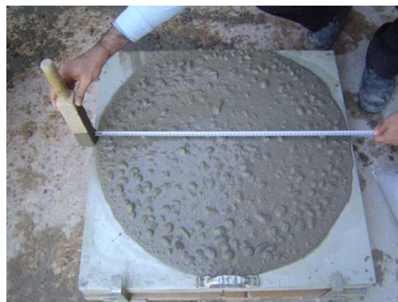
Figure 7. Slump flow spread
